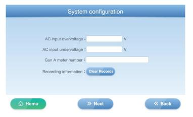
AC input undervoltage: According to the system voltage setting of the power supply, the default setting is 330V
