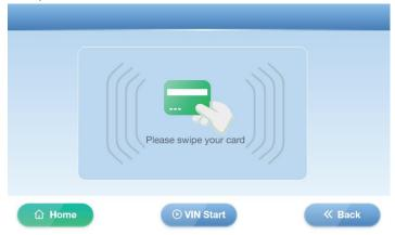
2) After swiping the card, the charging station automatically detects for a few seconds and starts charging. The charging interface displays information such as Battery SOC, Charging time, Card Balance, Charging current, Amount charged, Battery type, Charging voltage, etc.
