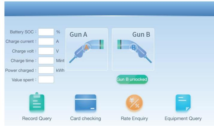
The charging interface displays information such as Battery SOC, Charging current, Charge volt, Charging time, Power charged, Value spent, etc.
