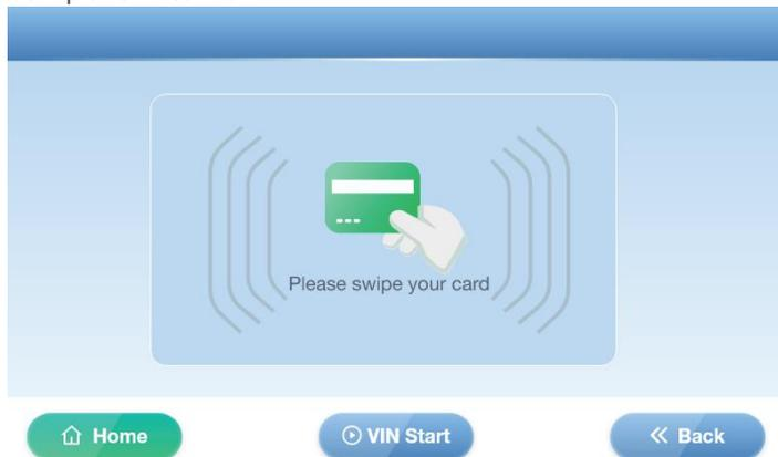
2) After swiping the card, the charging station automatically detects for a few seconds and starts charging. The charging interface displays information such as Battery SOC, Charging time, Card Balance, Charging current, Amount charged, Battery type, Charging voltage, etc.
