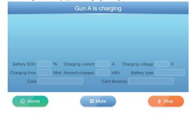
3) The network starts charging, and the charging station automatically detects for a few seconds before starting charging. The charging interface displays information such as Battery SOC, Charging current, Charge volt, Charging time, Power charged, Value spent, etc.
