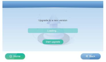
then insert the USB drive containing the program into the USB interface of the charging station motherboard. Click the Start upgrade button to start upgrading the program. The progress bar at the bottom reaches the far right, and the upgrade is completed. Restart the charging station.
