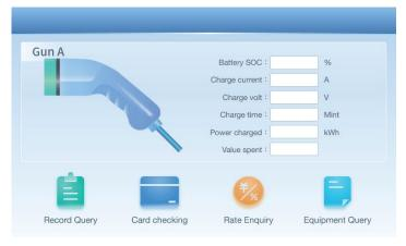
displays information such as Battery SOC, Charging current, Charge volt, Charging time, Power charged, Value spent, etc.
